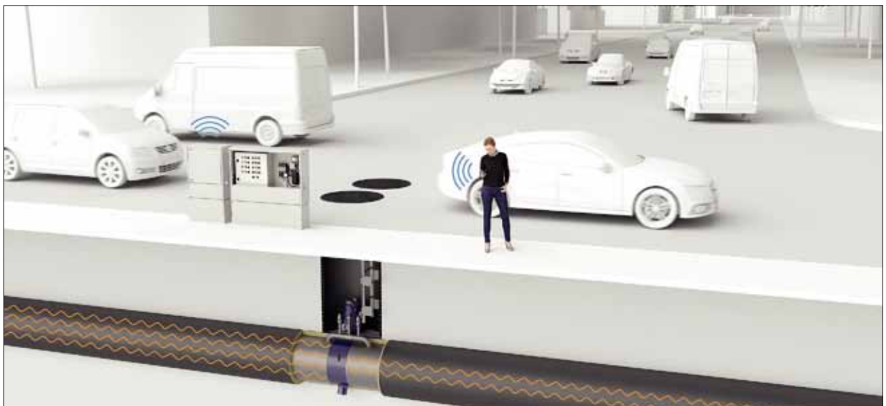
Figure 3. The hydraulic valve operation solution combined with a plastic access chamber is just one example of the kind of solutions that are going to be essential for future Smart Cities
